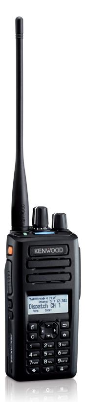
This versatile handheld radio supports both NXDN and DMR digital protocols as well as mixed digital & FM analog operation, enabling it to serve with distinction in a wide range of enterprise- and operation-critical applications. Compact yet designed with durability in mind, it's packed with convenient features like Bluetooth® for hands-free operation and built-in GPS. Additionally, for expansion capability a software license certification system facilitates extensive customization.
